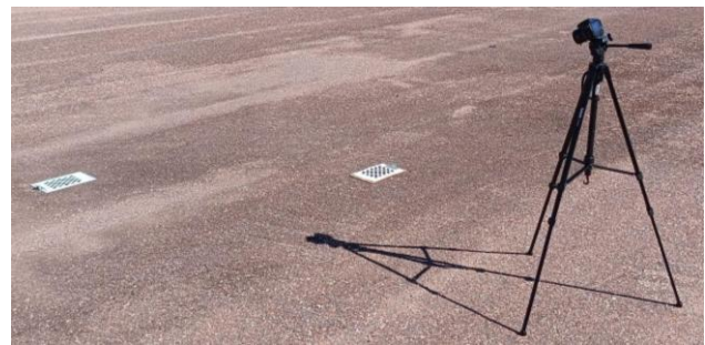
Figure 11. Layout of the camera, tripod and chessboard templates.
