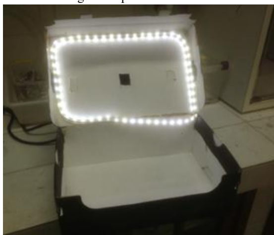
Figure 3. Optical box with its lid opened and LED lights on.
